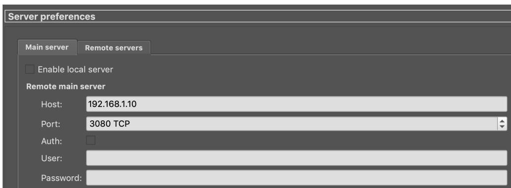
Just indicate the IP address of the server that runs GNS3 virtual machine.
