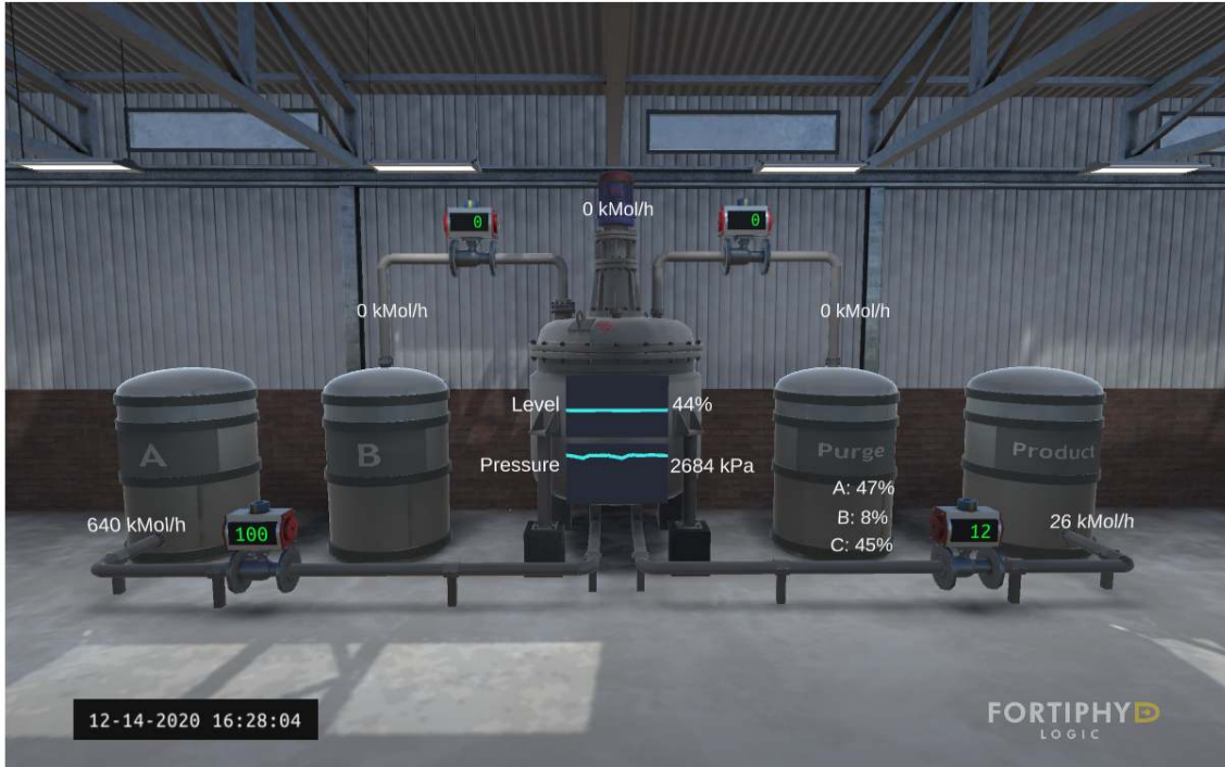
Figure 6.1: GRFICSv2 visual simulation of chemical process
